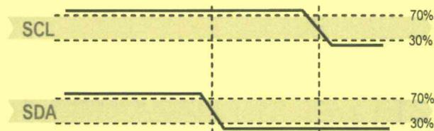
**Figure 13** Transmission Start condition (S) - a high to low transition on the SDA line while SCL is high. The Start condition is a unique state on the bus created by the master, indicating to the slaves the beginning of a transmission sequence (bus is considered busy after a Start).
