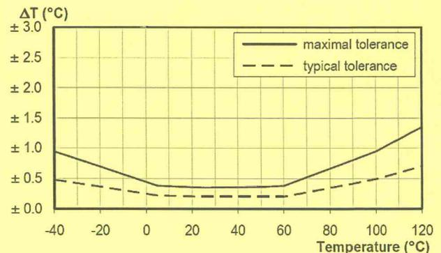
Figure 3 Maximal tolerance for temperature sensor in °C.
