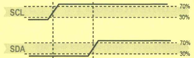
**Figure 14** Transmission Stop condition (P) - a low to high transition on the SDA line while SCL is high. The Stop condition is a unique state on the bus created by the master, indicating to the slaves the end of a transmission sequence (bus is considered free after a Stop).
