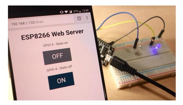
This ESP8266 Web Server is mobile responsive and it can be accessed with any device that as a browser in your local network. The code for this project is done using Arduino IDE.
